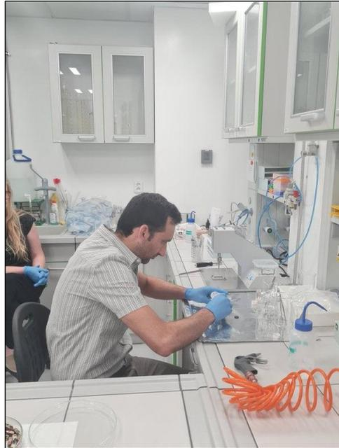
***Figure 37 – Students preparing sample for AMS measurement using pneumatic sample press.***
